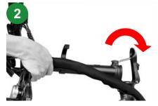
Open the quick release on the standpipe. Thread the handlebar into the standpipe.
