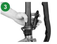
Press the folding buckle to secure the folding handlebar.
