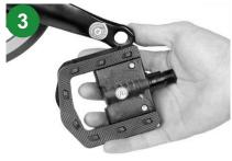
Locate the corresponding pedal according to the label. Right pedal: Rotate clockwise. Left pedal: Rotate counterclockwise.
