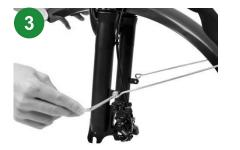
Unscrew both sides of the front fork. Install the fender bracket on both sides of the front fork.
