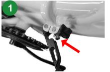
There's a screw that prevents the buckle from closing, You need to adjust the screw into correct angle manually.
