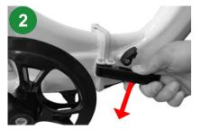
Use your finger to hook the small lever and rotate it upwards.
