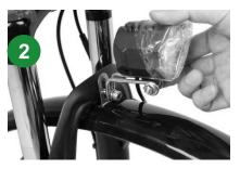
Remove the screw from the front fork. Screw as shown in the picture through the gasket, headlight, fender to assemble.
