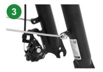
Unscrew both sides of the front fork. Install the fender bracket on both sides of the front fork
