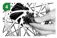
Remove the nuts and water drop gaskets on both sides of the front wheel.
