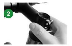
Insert the handle bar into the fork locknut to the desired height. Place the handlebar on the stem correctly.
