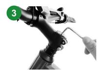
Center the handlebar and adjust the direction, Make sure the handlebar is centered on the stem.
