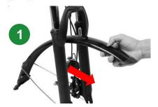
The fender follows the direction of the arrow through behind the front fork. Avoid fender brackets that fail to reach the correct position.
