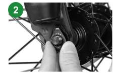
Hang the water drop gasket hook facing up on both sides of the front fork. Then install the nuts on both sides of the axle.
