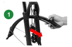
The fender follows the direction of the arrow through behind the front fork. Avoid fender brackets that fail to reach the correct position.
