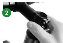
Insert the handle bar into the fork locknut to the desired height. Place the handlebar on the stem correctly.
