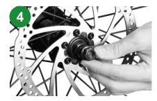
Remove the nuts and water drop gaskets on both sides of the front wheel.
