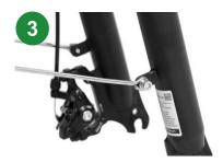
Unscrew both sides of the front fork. Install the fender bracket on both sides of the front fork.
