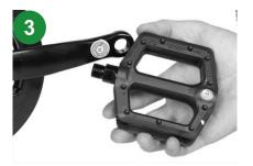
Locate the corresponding pedal according to the label. Right pedal: Rotate clockwise. Left pedal: Rotate counterclockwise.
