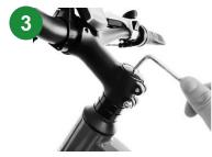
Center the handlebar and adjust the direction, Make sure the handlebar is centered on the stem.
