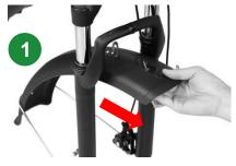
The fender follows the direction of the arrow through behind the front fork. Avoid fender brackets that fail to reach the correct position.
