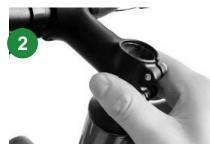
Insert the handle bar into the fork locknut to the desired height. Place the handlebar on the stem correctly.
