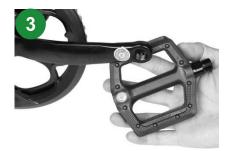
Locate the corresponding pedal according to the label. Right pedal: Rotate clockwise. Left pedal: Rotate counterclockwise.
