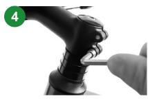
Use the wrench to tighten the screw and fix the handlebar stem in place, Check it again to make sure the handlebar stem is in line with the toptube, then use the wrench to tighten the screw and fix the handlebar stem in place.
