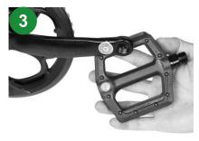
Locate the corresponding pedal according to the label.
