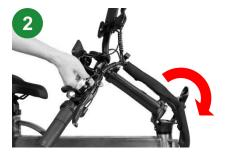
Open the fold of the handlebar up.
