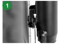
Attach the tire to the front fork. Make sure the brake disc goes through the gap in the middle of the brake
