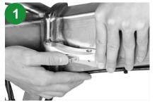
Press the front end of the buckle with your left hand. Push the button forward with your right thumb.
