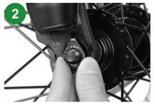
Hang the water drop gasket hook facing up on both sides of the front fork. Then install the nuts on both sides of the axle.
