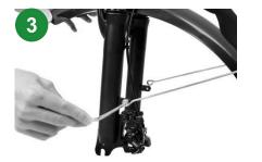
Unscrew both sides of the front fork. Install the fender bracket on both sides of the front fork.
