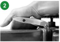
After the screw rod is pushed in, press the folding buckle inward to complete the closing
