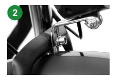
Remove the screw from the front fork. Screw as shown in the picture through the gasket, headlight, fender to assemble.
