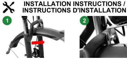
The fender follows the direction of the arrow through behind the front fork. Avoid fender brackets that fail to reach the correct position.
