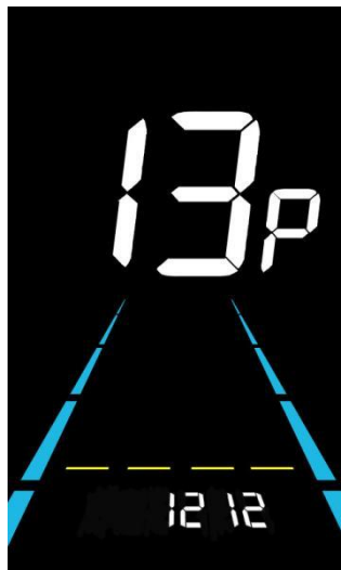
Figure 6-16 Power-on password setting interface
